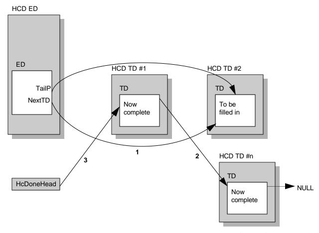
Figure 5-8: Host Controller Removes a Transfer Descriptor from a Queue
