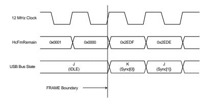
Figure 6-2: Timing for SOF Token Generation on USB
