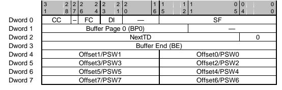
Figure 4-3: Isochronous TD Format
