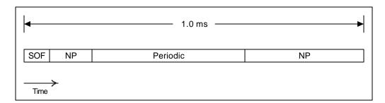
Figure 3-6: Frame Bandwidth Allocation
