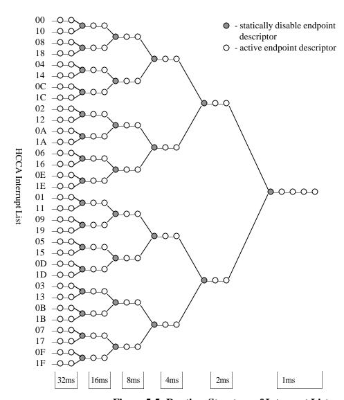
**Figure 5-5: Runtime Structure of Interrupt Lists**
