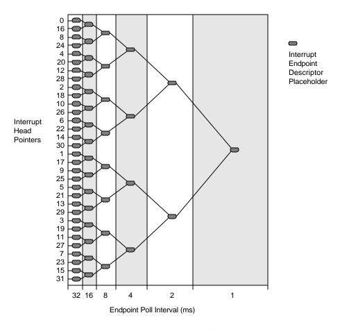
Figure 3-4: Interrupt ED Structure
