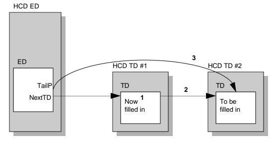
Figure 5-7: Adding a Transfer Descriptor to a Queue
