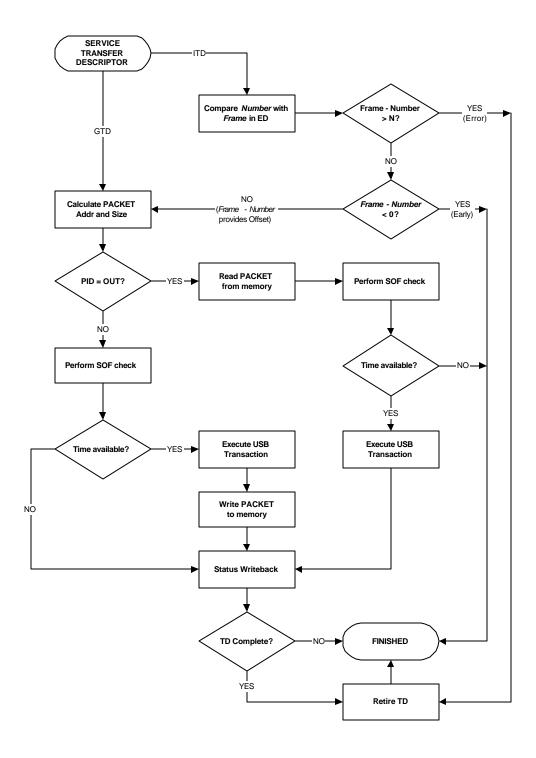
Figure 6-7: Transfer Descriptor Service Flow
