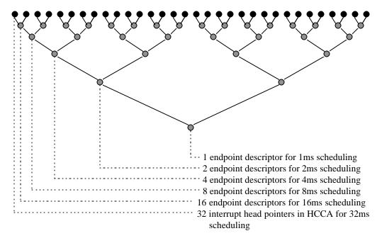
Figure 5-4: Structure of Interrupt Lists
