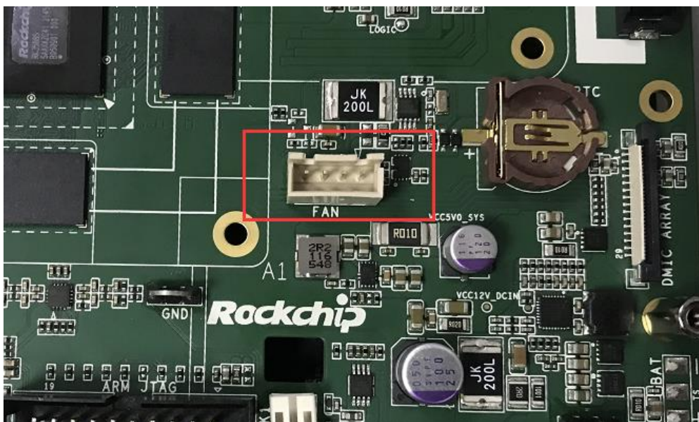
Figure 3-7 Fan Power Interface
