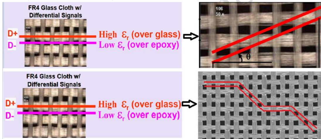
Figure 3-63 PCB fiberweave effect to improve routing way
