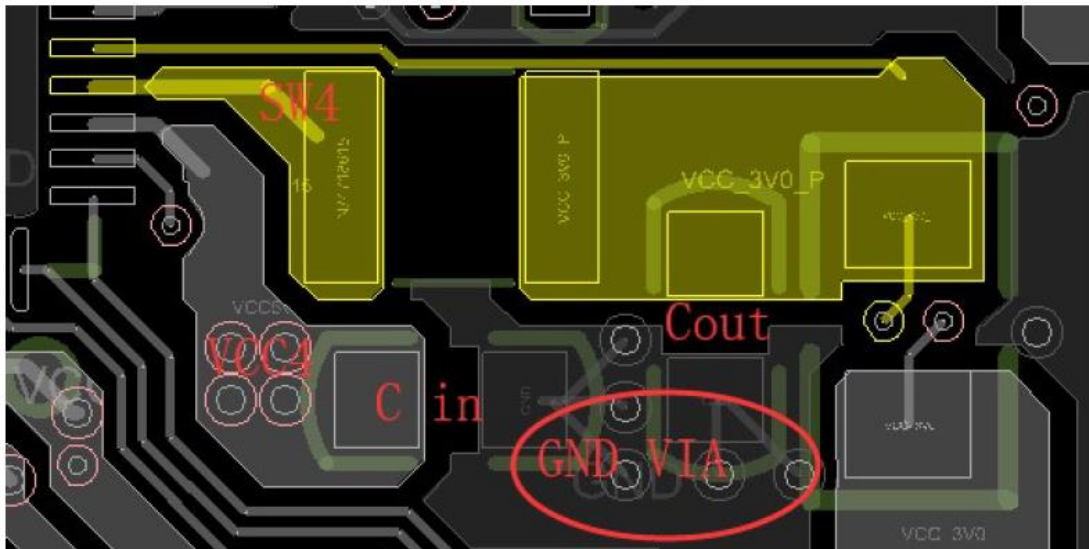
Figure 3-15 RK809-5 BUCK4 Layout and routing
