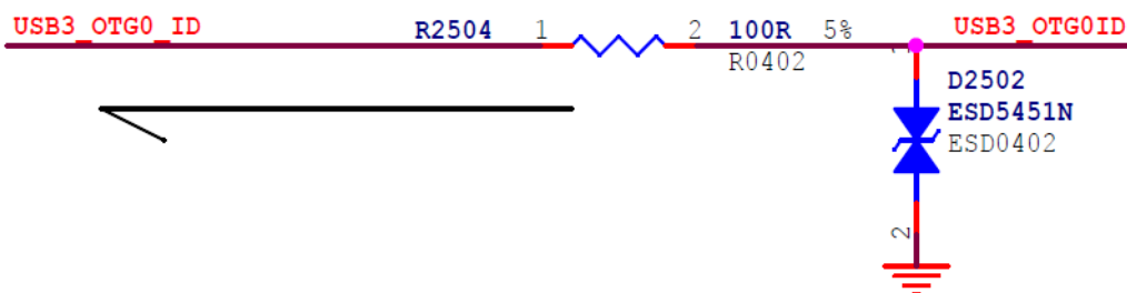
Figure 2-87 USB OTG ID pin circuit
