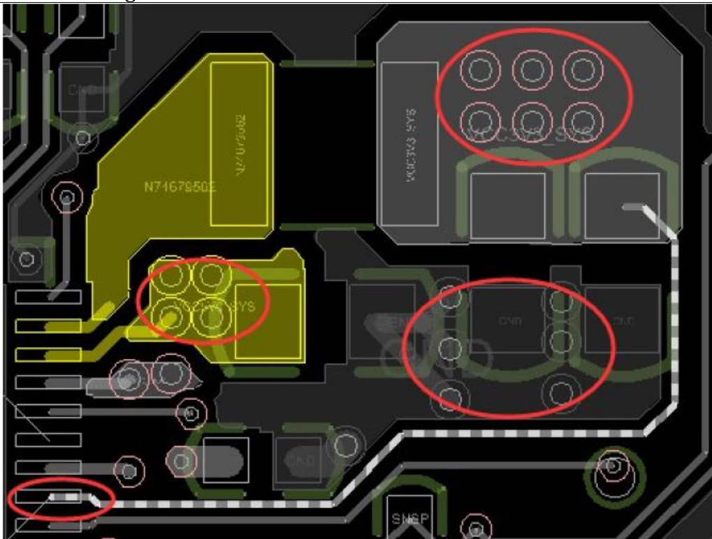
Figure 3-16 RK809-5 BUCK5 Layout and routing
