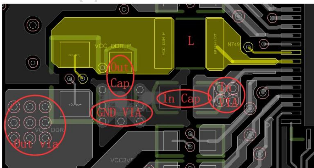
Figure 3-14 RK809-5 BUCK3 Layout and routing
