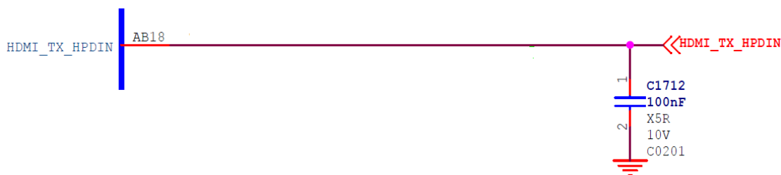
Figure 2-116 RK3568 HDMI2.0 TX PHY HPD pins
