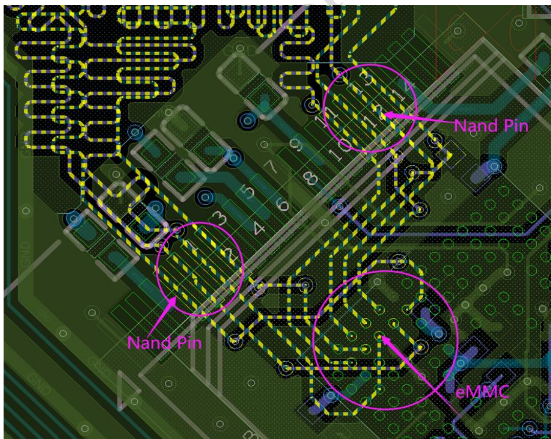
Figure 3-61 DATA routing of eMMC and Nand Flash compatible design
