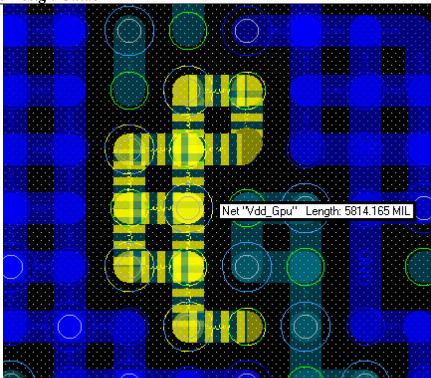
Figure 3-27 RK3568 VDD_GPU Power pin traces and vias
