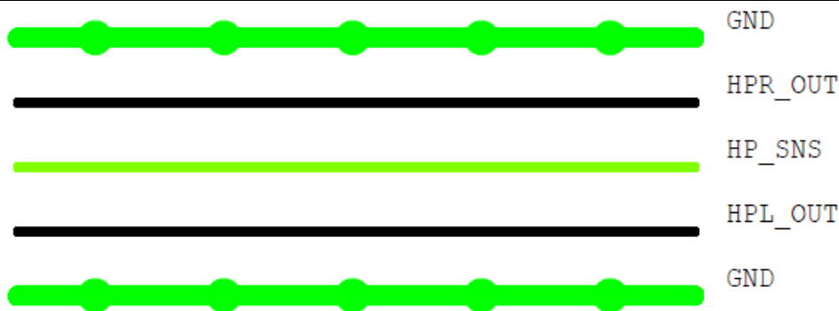
Figure 2-153 RK809 Codec output earphone circuit
