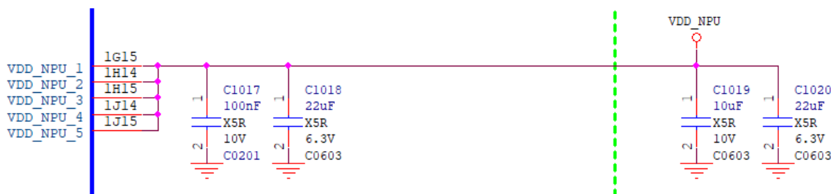
Figure 2-22 RK3566 VDD_NPU power and decoupling
